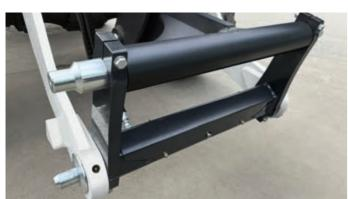
Quicktach coupler (installed as standard)
