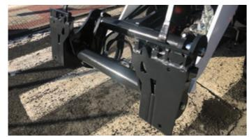
Quick-Tach $^{\text{TM}}$  to Bob-Tach $^{\text{TM}}$  adapter (required for all attachments except buckets and pallet forks)
