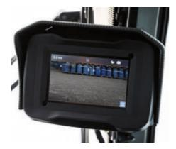
The jog shuttled-controlled LCD screen displays critical updates and automatically switches to the rear-view camera's feed when in reverse.
