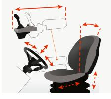
Easily adjust the position of the steering wheel, joystick and seat to what suits you best. Make your loader fit you like a glove.
